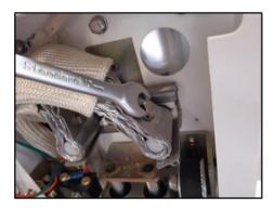
**2. Unscrew the braided alum. conductor** from the rod with a wrench.
