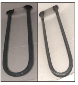
Example of rods after decontamination
